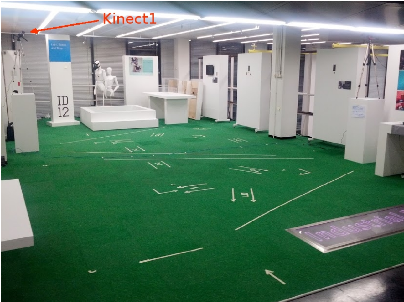
Figure 8. The experiment venue. Markers on the floor indicate the start and end points and numbered reference points for standing in a predefined orientation. Additional markers also show which part of the area is covered by which Kinect device.
