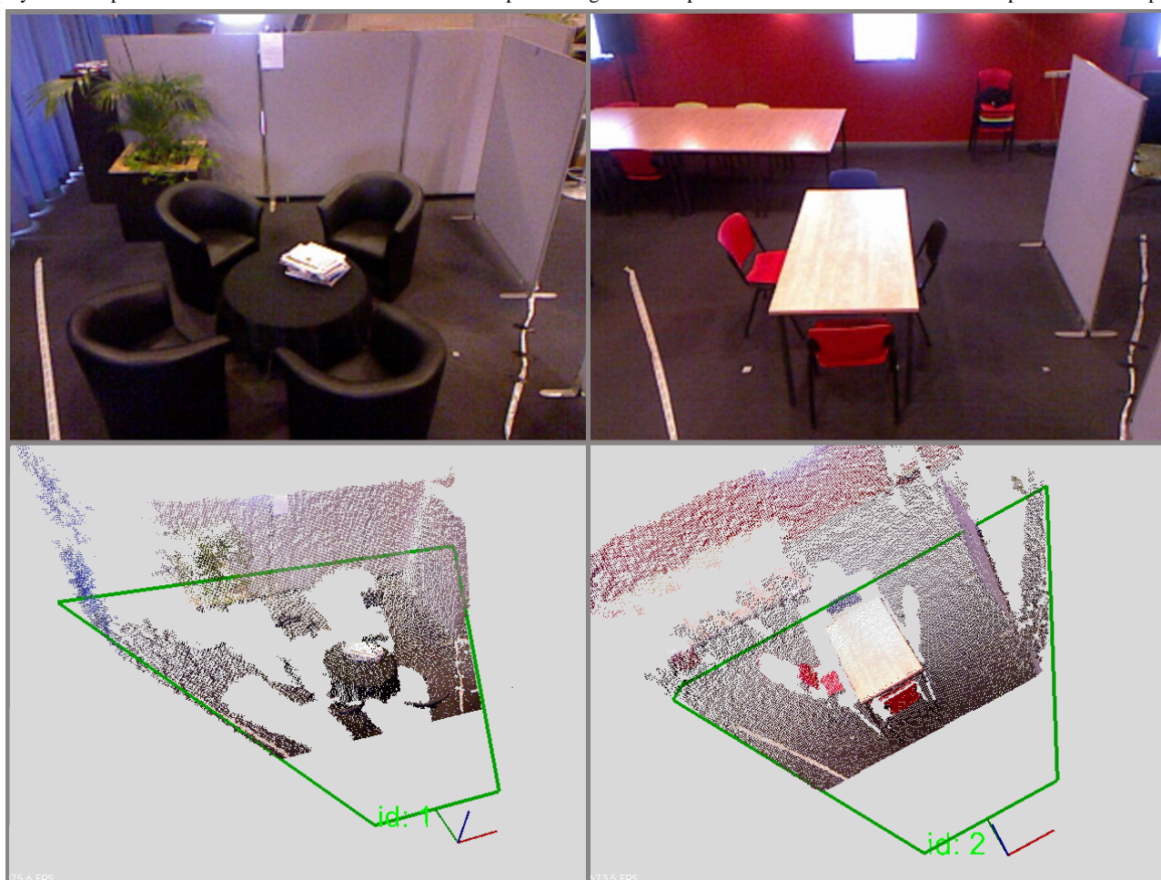
Figure 2. Example of a test bed with two scenes being independently covered by Kinect sensors. Mock-up of a living room on the left and a dining room on the right. Images in the top row depict the point-of-view of the cameras when they are mounted in the overhead position. The bottom row displays colored point clouds of scenes that are obtained from depth sensing. Green trapezoid indicates the area in which it is possible to track people.
