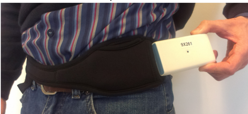
Figure 1. Portable inertial sensor and the neoprene belt where the sensor was inserted.
