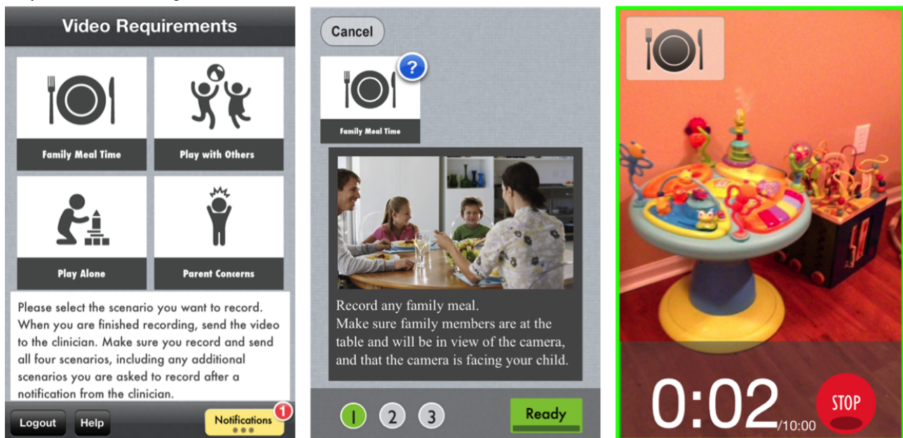
Figure 2. NODA smartCapture. (1) Home screen showing 4 NODA scenarios, as well as status of ones recorded. (2) Each scenario has recording instructions for parents as prescription. Pressing “Ready” proceeds to recording interface. (3) Recording mode with clear time-elapsed status and a green boundary to reinforce recording mode.
