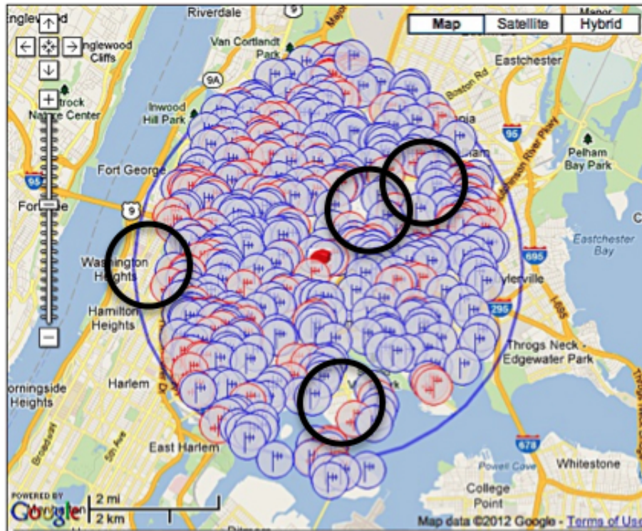
Figure 7. Antenna sites: Bronx Borough, New York. Black circles indicate gaps in service.
