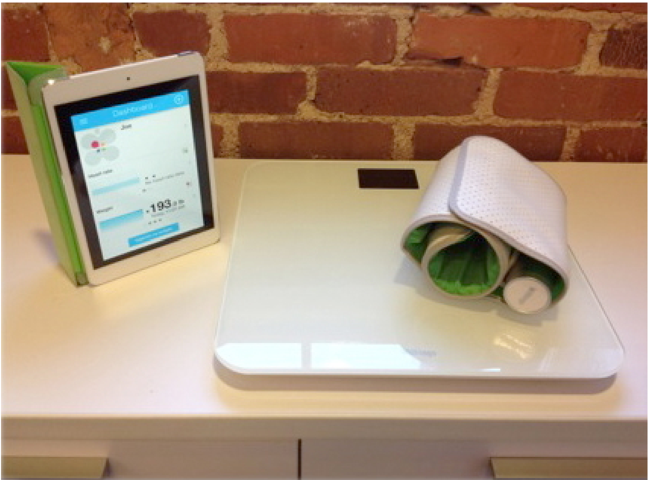
Figure 1. Portable devices provided to participants as part of the intervention (from left: iPad Mini, bluetooth weight scale, auto-inflating blood pressure cuff).
