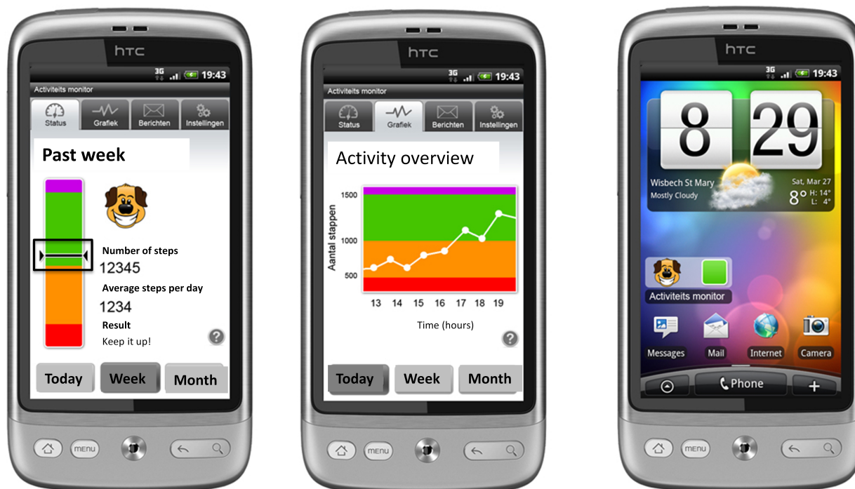
Figure 4. In version 3, the bar on the left side combines amount and intensity of steps. The DPA goal is met when the vertical stripe (representation of current activity status) is kept in the rising rectangle at all times until the green area is reached. Absolute number of steps and current advice on DPA progress are also shown (pilot study C3).
