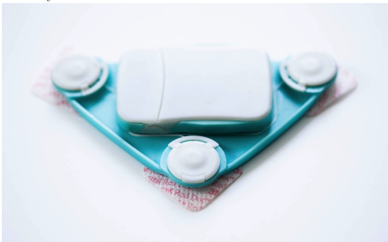
Figure 2. Final design of the Beat wearable ECG sensor with electrodes attached.
