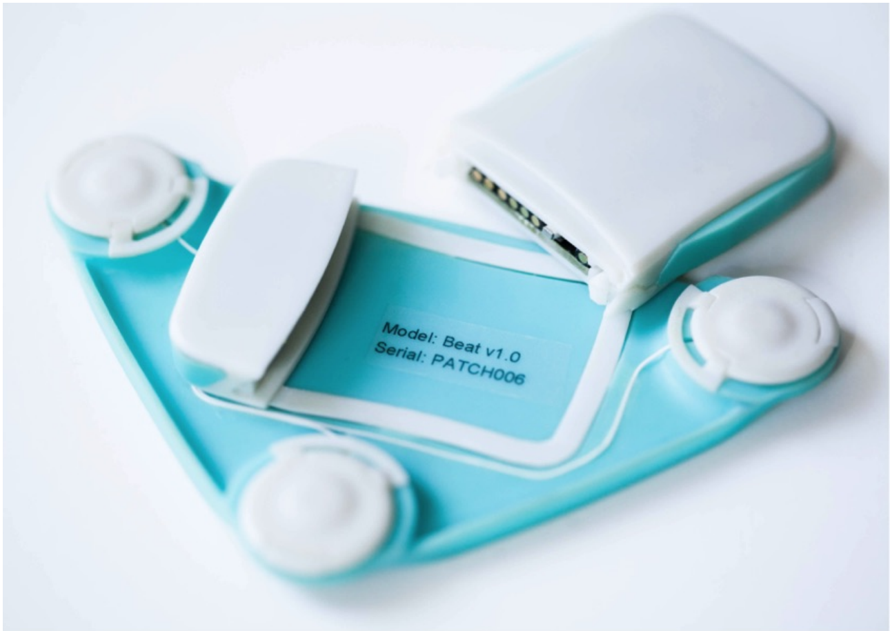
Figure 3. Individual components of the Beat wearable ECG sensor showing the electronics module and patch module.
