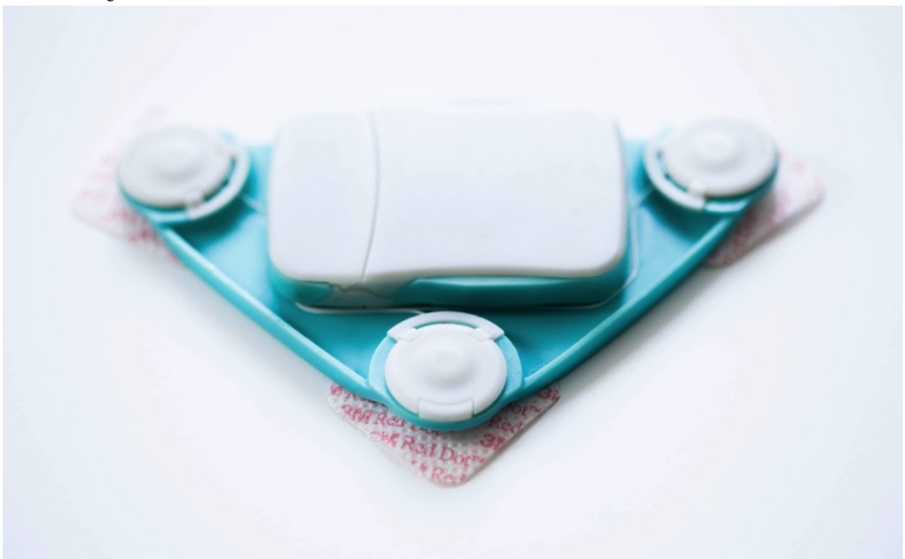
Figure 2. Final design of the Beat wearable ECG sensor with electrodes attached.
