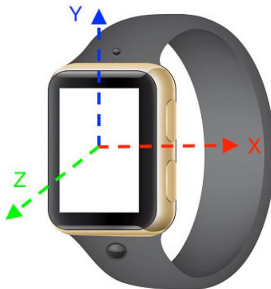
Figure 1. An illustration of accelerometer axes on a typical smartwatch.
