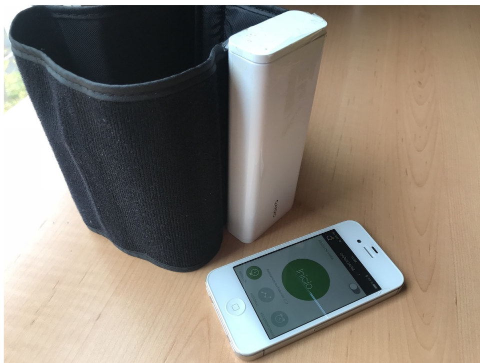
Figure 1. QardioArm is a device with a cuff used with an app for visualization of blood pressure known as Qardio.
