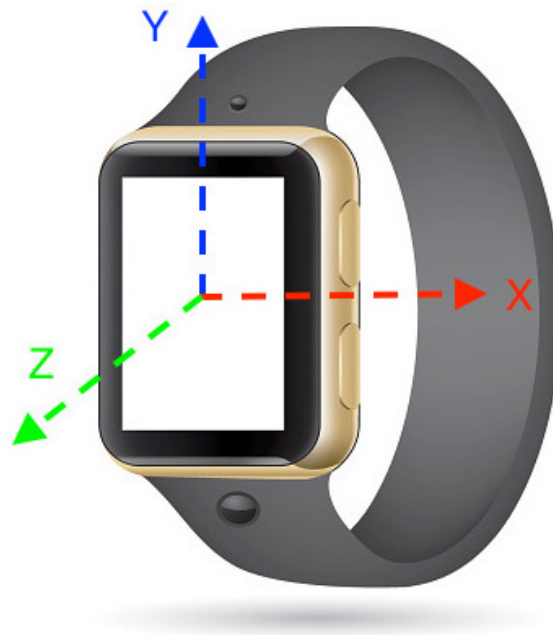
Figure 1. An illustration of accelerometer axes on a typical smartwatch.
