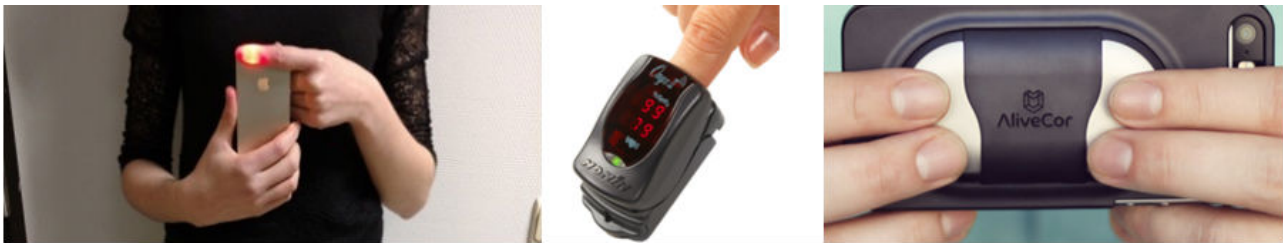
Figure 4. Graphical representation of how measurements are performed using the different devices. Left, FibrCheck application; Middle, Nonin oximeter; Right, AliveCor.
