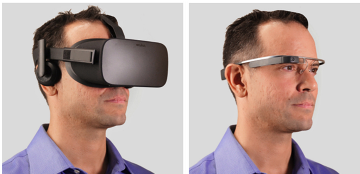
Figure 6. Fully immersive head-mounted device compared with partially immersive smartglasses. Fully immersive virtual reality headsets, such as Oculus Rift (left), completely block external stimuli, limiting their use in concussed populations where dizziness, nausea, and sensitivity to light are common persistent symptoms. Smartglasses, such as Glass (right), could provide a safer, more portable, and lighter-weight alternative. Of note, Glass weighs only 1.3 ounces—more than 10 times less than Oculus Rift.
