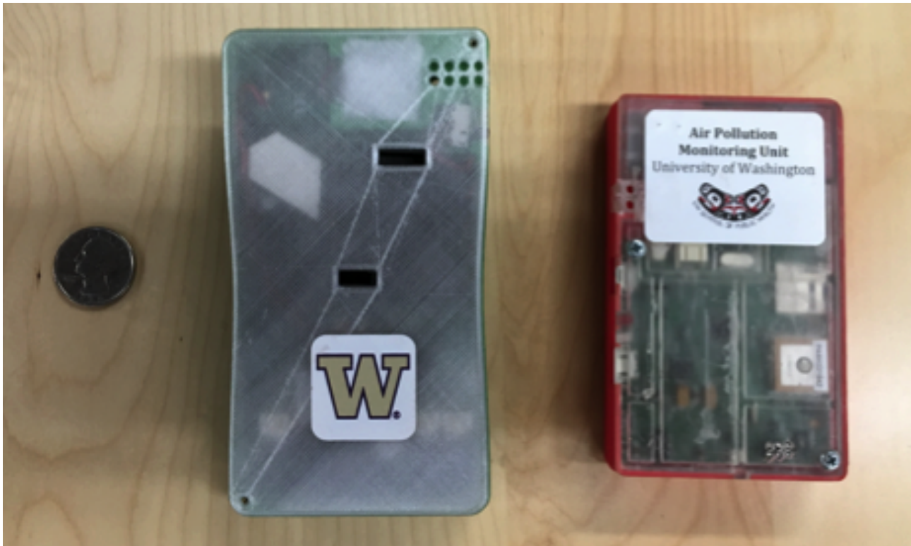
Figure 1. Size comparison of a personal air pollution monitor in cycle 2 (left) to cycle 3 (right) of the design feedback iterative cycle.
