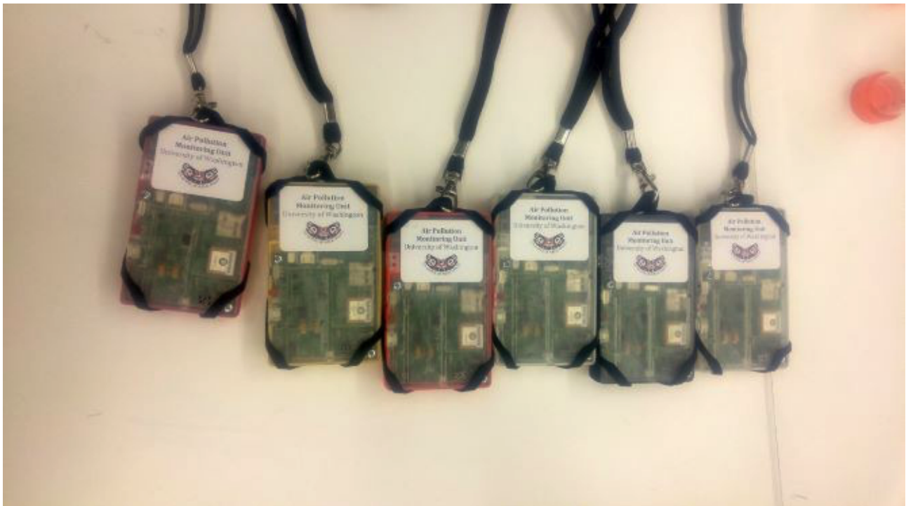
Figure 2. Lanyards were used in cycle 3 to allow participants to carry the air pollution monitor around the neck or attached to a bag.
