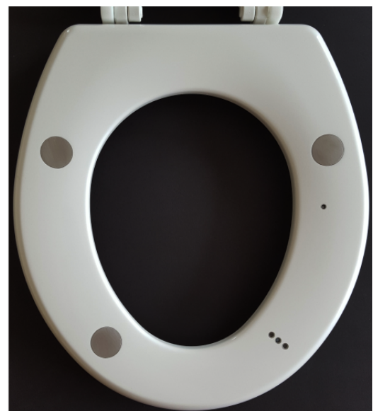
Figure 1. Stainless-steel electrodes are integrated into the seat and are connected directly to the integrated ECG analog front-end. The output of each front-end is low-impedance, allowing for a low-noise connection to the differential ECG amplifier inside of the BIOPAC MP150 system (left). The resulting full-scale ECG signal is acquired on a NI CompactRIO DAQ. For the HF subject study, all instrumentation and data acquisition circuitry are integrated into the toilet seat (right). DAQ: data acquisition system; ECG: electrocardiogram; bECG: buttocks ECG; NI: National Instruments; HF: heart failure.
