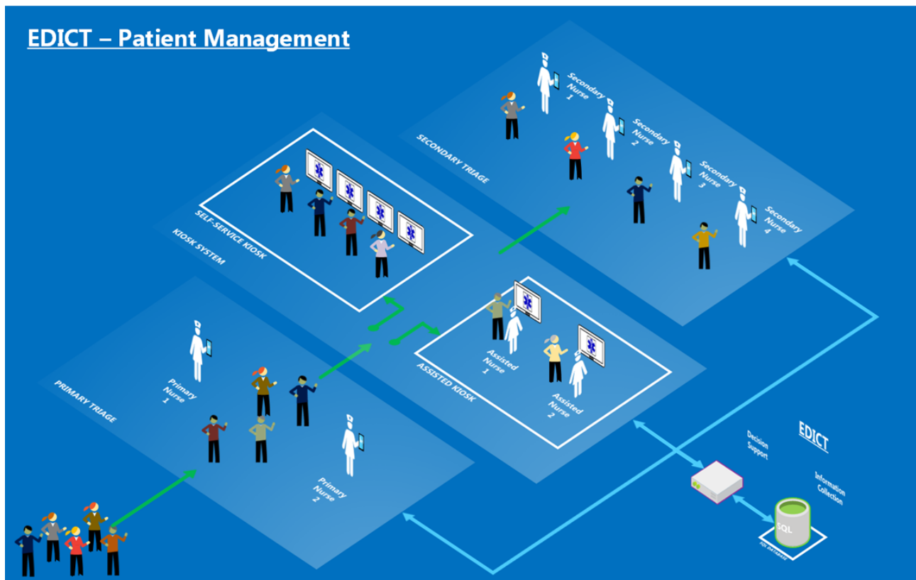
Figure 11. EDICT, a mass casualty incident–specific triage tool used to map data gathered by the mobile application to the Irritant Gas Syndrome Agent algorithm. Information gathered in the primary triage, the kiosk system and secondary triage is used to determine a patient's specific exposure level and action.
