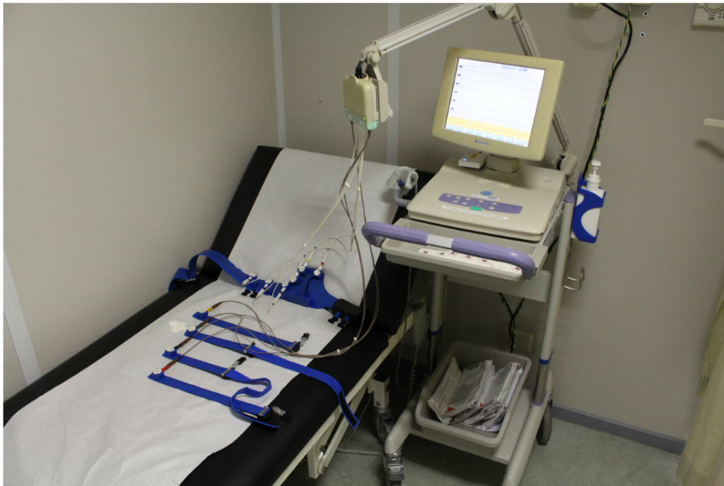
Figure 12. Detailed picture of the prototype (blue) connected to the standard electrocardiogram monitoring equipment. Note that in the final design, the electrode wires will be integrated into the belt.
