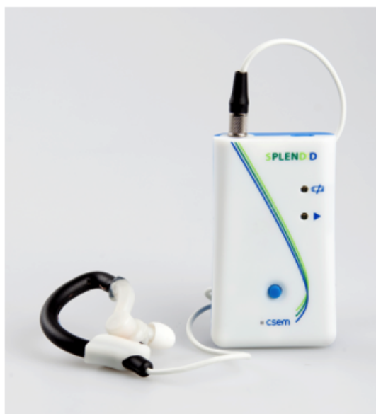
Figure 5. Integrated version of the SPLENDID eating detection sensor with its datalogger.
