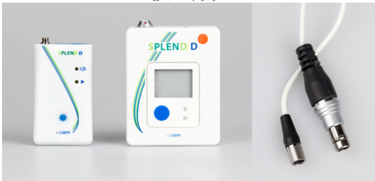
Figure 6. Old version and new, smaller version of the datalogger (left) and plug (right).
