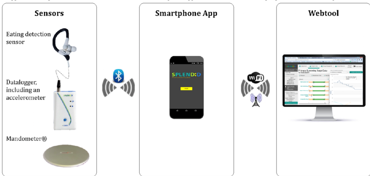
Figure 1. The SPLENDID eating detection sensor integrated into the full SPLENDID system. This system combines the eating detection sensor with a datalogger (including an accelerometer), the Mandometer, a smartphone app, and a webtool, functioning together as a “wearable personal coach.”.
