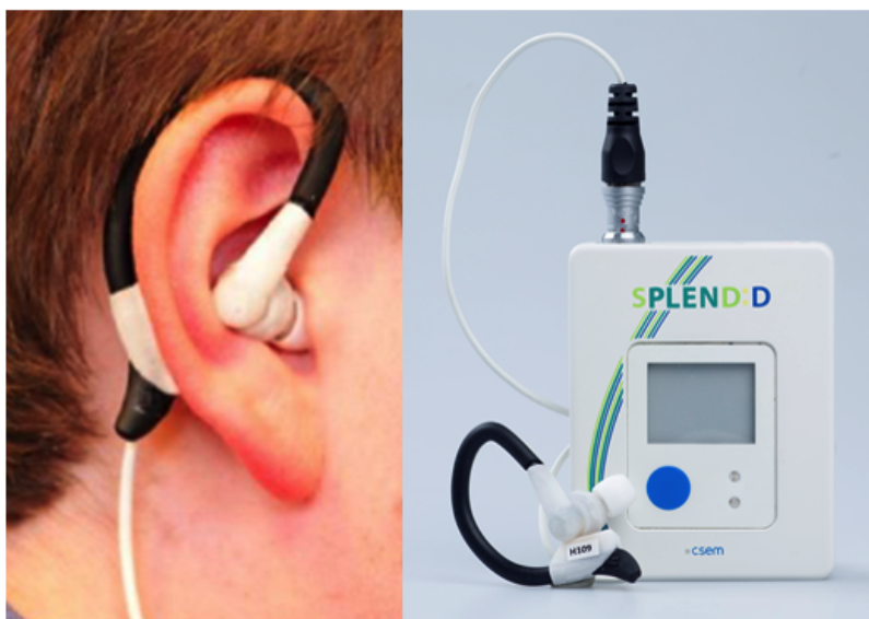
Figure 4. First wearable version of the eating detection sensor (left: the eating detection sensor; right: the eating detection sensor and the datalogger).
