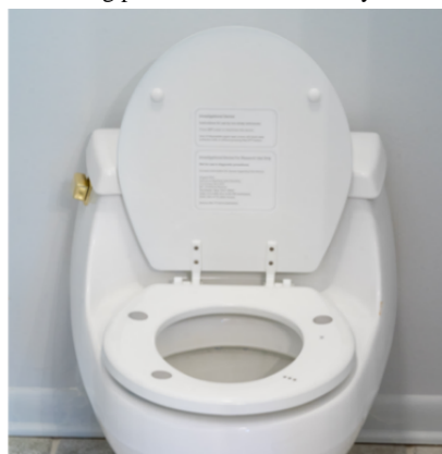
Figure 1. A toilet seat-based cardiovascular monitoring system (left) is integrated into an individual’s daily routine without requiring any change in habit, thereby addressing patient adherence. The system captures a comprehensive set of clinically relevant measurements automatically (right).
