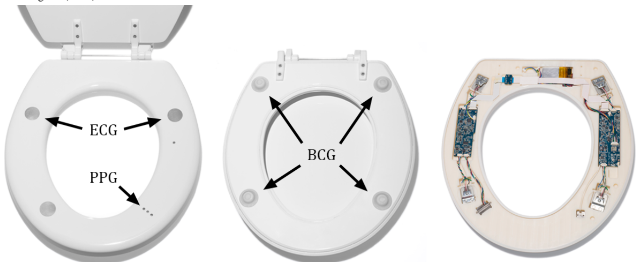
Figure 2. The toilet seat-based cardiovascular monitoring system is completely self-contained, battery-powered, wireless, and cleanable with all sensors and electronics instrumentation integrated inside of the seat. It can measure the electrocardiogram (ECG), photoplethysmogram (PPG), and the ballistocardiogram (BCG).
