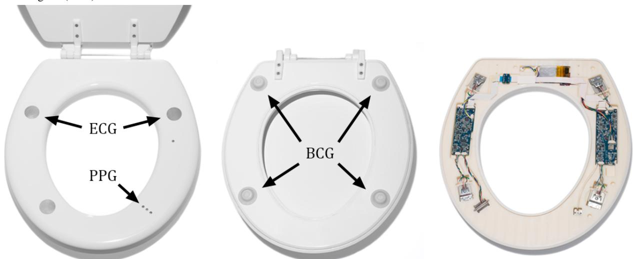
**Figure 3.** A floating hinge ensures that the weight on the seat is completely captured by the load cells under each standoff rather than having a portion of it carried by the hinge. This is a requirement for accurate ballistocardiogram monitoring on a toilet seat.
