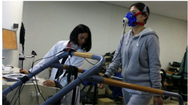
Figure 1. Illustration of the foot monitoring system (left) and a picture of a participant walking on an uphill treadmill wearing the K4b2 portable gas analyzer (right).
