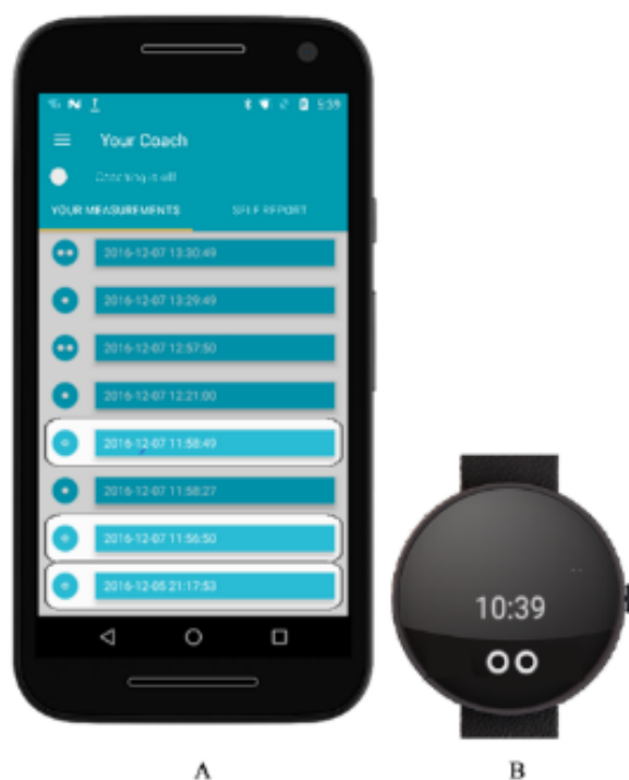
Figure 6. Examples illustrating the visualization of the low-arousal state “hollow spheres” on the smartphone (A) and smartwatch (B) interface.
