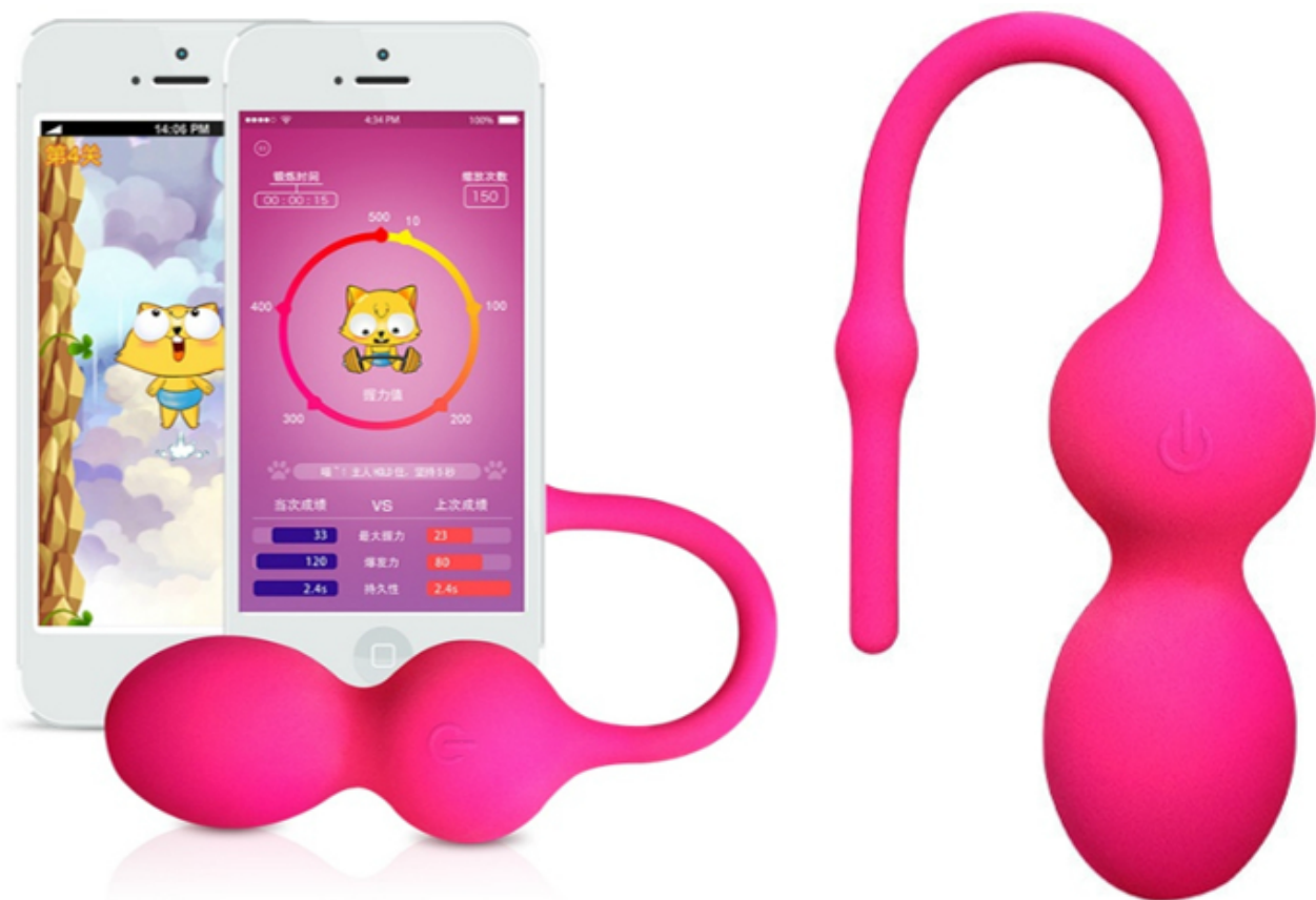
Figure 1. The mHealth iBall device. The iBall device consists of a Bluetooth antenna that sits outside of the body and 2 spherical compartments containing a battery and biofeedback sensor that sits within the vaginal canal.
