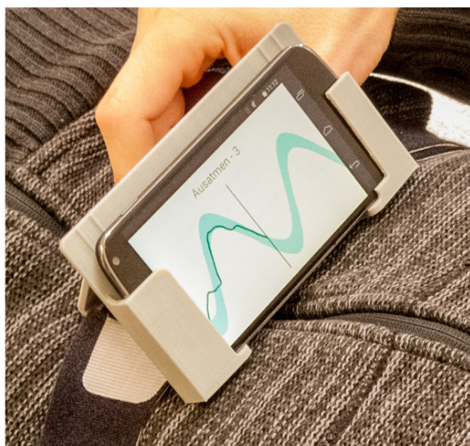
Figure 1. The Breathing-Mentor training user interface combines graphical (moving sine wave) and text instructions (inhale/exhale, counting from 1 to 4) for deep, slow abdominal breathing with biofeedback (dark line, not present in the control version).
