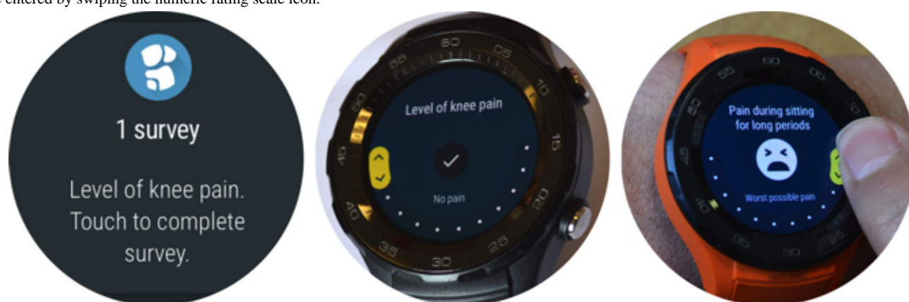
Figure 1. User interface of KOALAP app. Left: notification of an active survey; middle: data entry screen for survey “level of knee pain”; right: data are entered by swiping the numeric rating scale icon.
