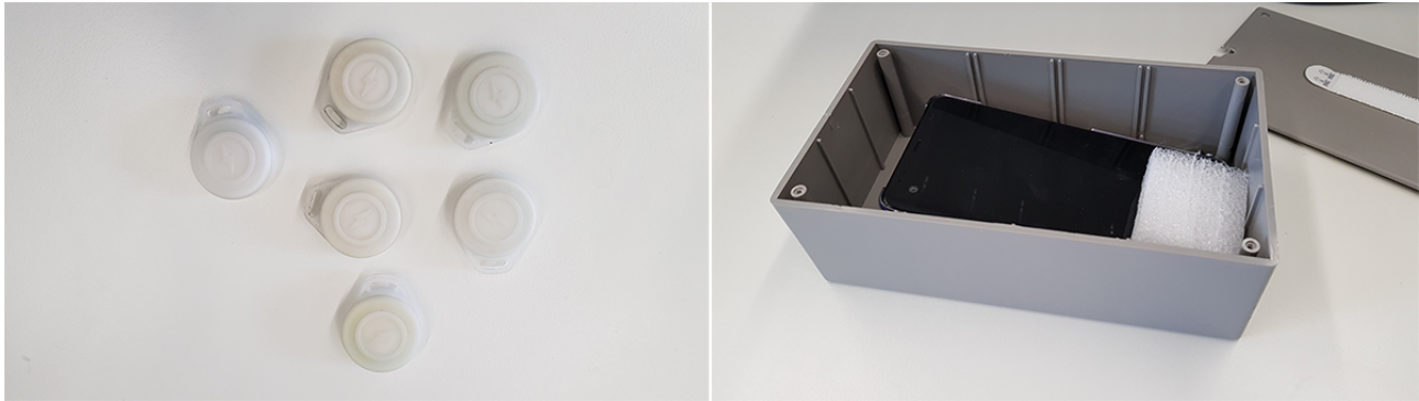
Figure 2. Beacons handed out to staff and patients; android devices that get mounted to the walls.
