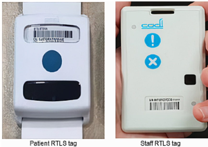
Figure 1. Mandatory real-time locating system (RTLS) tags worn by patients and staff within the vicinity of the COVID-19 screening centre for contact tracing purposes.
