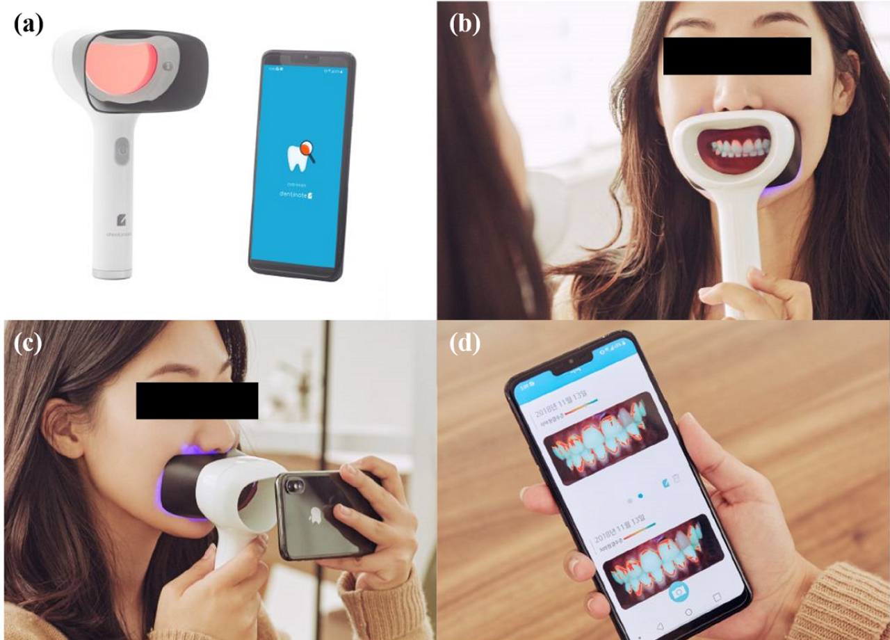
Figure 1. Oral hygiene monitoring system: (a) light-induced fluorescence device and hybrid mobile app; (b) method for monitoring oral hygiene with the naked eye through a mirror; (c) method for monitoring oral hygiene using smartphone; (d) hybrid mobile app that provides time series oral hygiene information.
