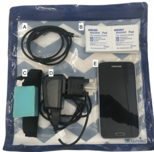
Figure 3. Equipment given to each study participant for the duration of the study: (A) 3.5-mm male-to-male TRRS audio cable, (B) Alcohol wipes, (C) NeMo device, (D) Smartphone charging cable with type-G adapter, and (E) Samsung Galaxy S5 smartphone.
