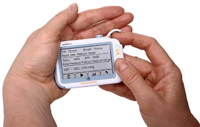
Figure 1. BodiMetrics Performance Monitor tricorder. Vital sign measurements are performed by placing the right index finger on the plethysmography sensor in the right upper corner under the flap. In addition, contact has to be made with the electrocardiogram electrodes at the front, left lateral side, and back using both hands.
