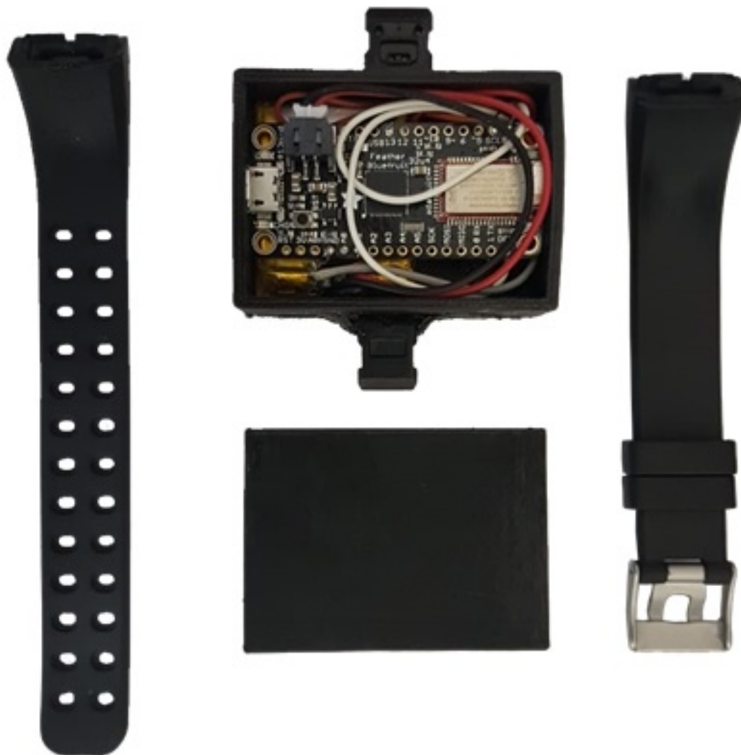
Figure 3. Prototype of the self-designed photoplethysmography sensor device.
