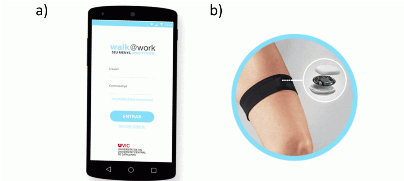
Figure 1. (A) Initial W@W-App interface and (B) the MetaWearC sensor with the waterproof case and the thigh band.
