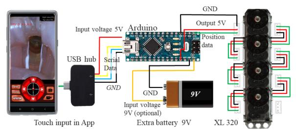
The microprocessor is connected to 4 motors, which are connected to wire-controlling pulleys. The motor (Dynamixel XL-320, Robotis) is a robot-exclusive smart actuator with a fully integrated direct current motor, reduction gearhead, controller, driver, and network in one direct current servo module [19]. Each motor has its own motor driver, allowing intuitive control by the microprocessor software.
