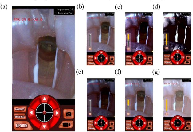
The app allows the user to capture the current view in two formats: as a still image and as a movie. The still capture button and video capture button at the bottom right of the screen perform this task. Image and videos are stored automatically in separate folders.
