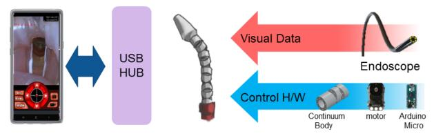
Through the OTG USB hub connection, the app, endoscope CMOS module, and microprocessor can interact with each other. Figure 2 presents a simplified circuit diagram of the device. With the OTG USB hub connection secured, the app obtains permission to access the camera and microprocessor. We used the Arduino Nano as a microprocessor, which is an open-source electronics platform, so that it can be easily used for
