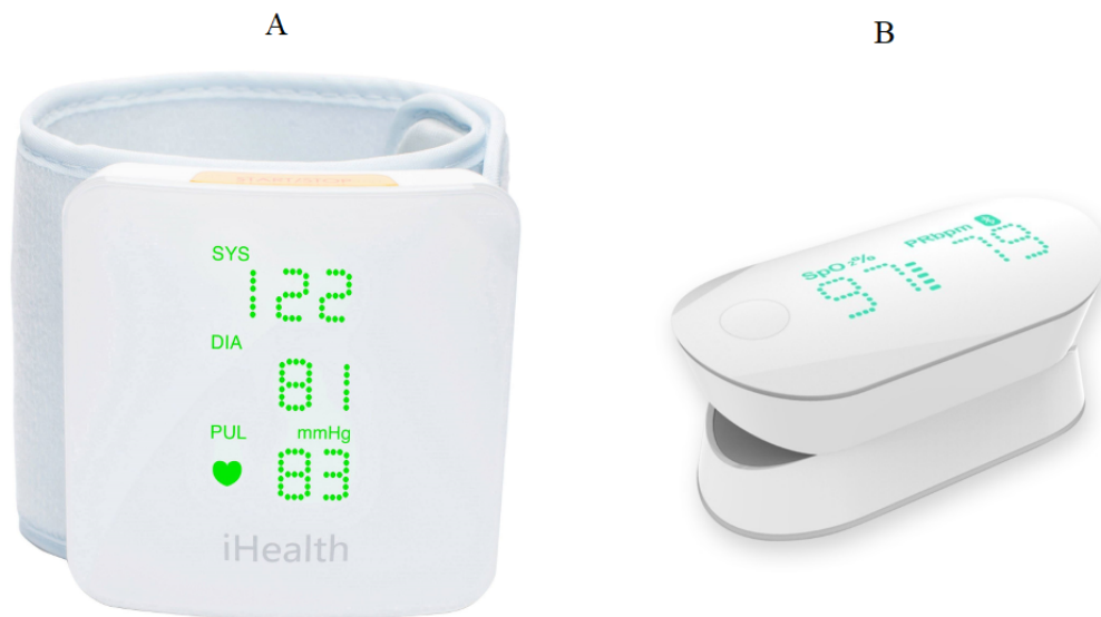
Figure 2. The devices used. (A) The wireless blood pressure wrist monitor (iHealth BP7). (B) The pulse oximeter (iHealth Oximeter PO3).
