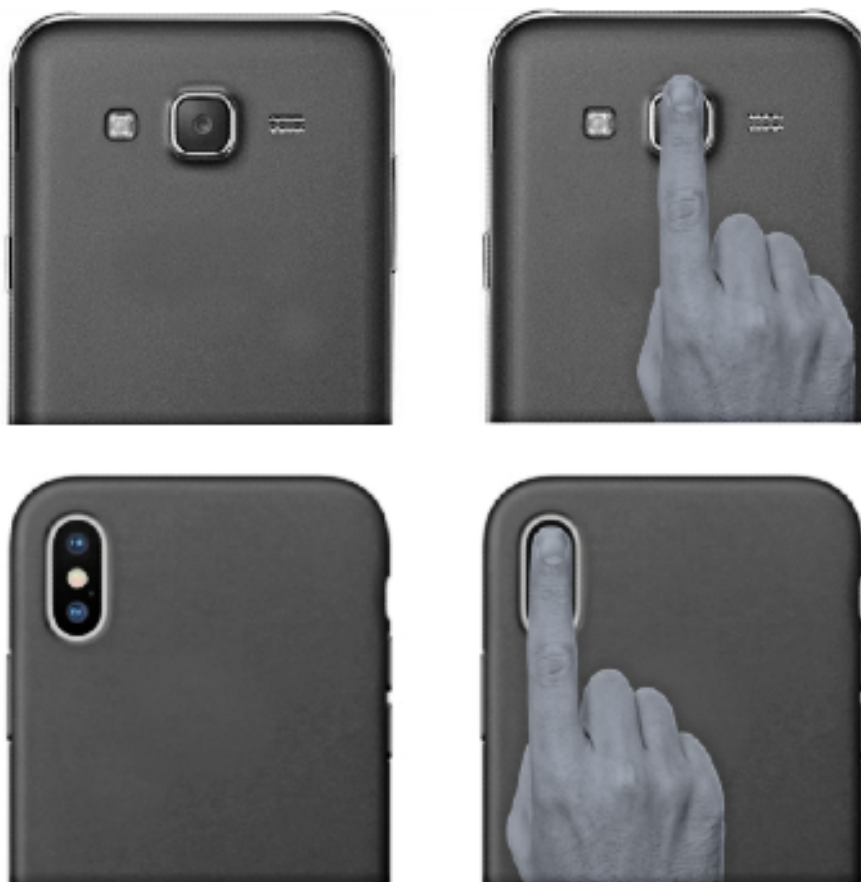
Figure 2. Correct placement of the index fingertip on different locations of the camera lens to obtain a correct heart rate measurement by photoplethysmographic imaging.
