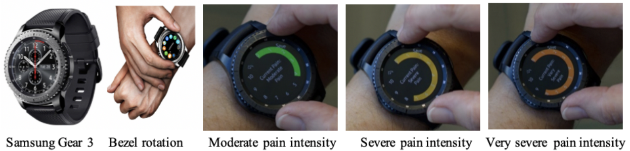
Figure 1. ROAMM app on Samsung Gear 3. Participants rotate the bezel on the watch to select the intensity on a scale from 0 to 10 and the color changes accordingly.
