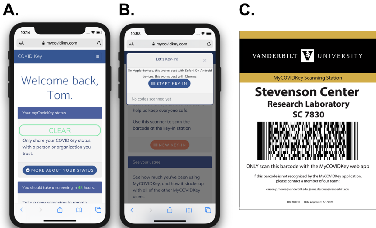
Figure 2. (A) The landing page of MyCOVIDKey, shown after a successful login. (B) A pop-up modal window that enables users to key in by scanning a location's bar code flyer. (C) A representative key-in flyer, with a barcode that has a unique embedded hash code specific to a location on campus.
