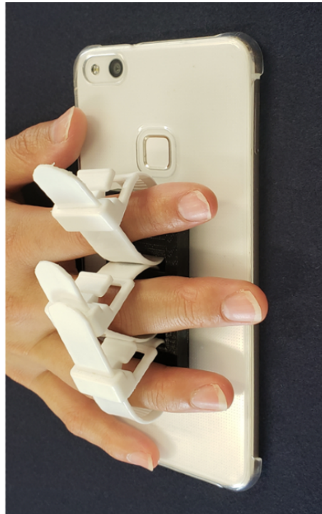
Figure 1. A finger guide attached to the back of the smartphone to fix the position of the fingers other than the thumb.
