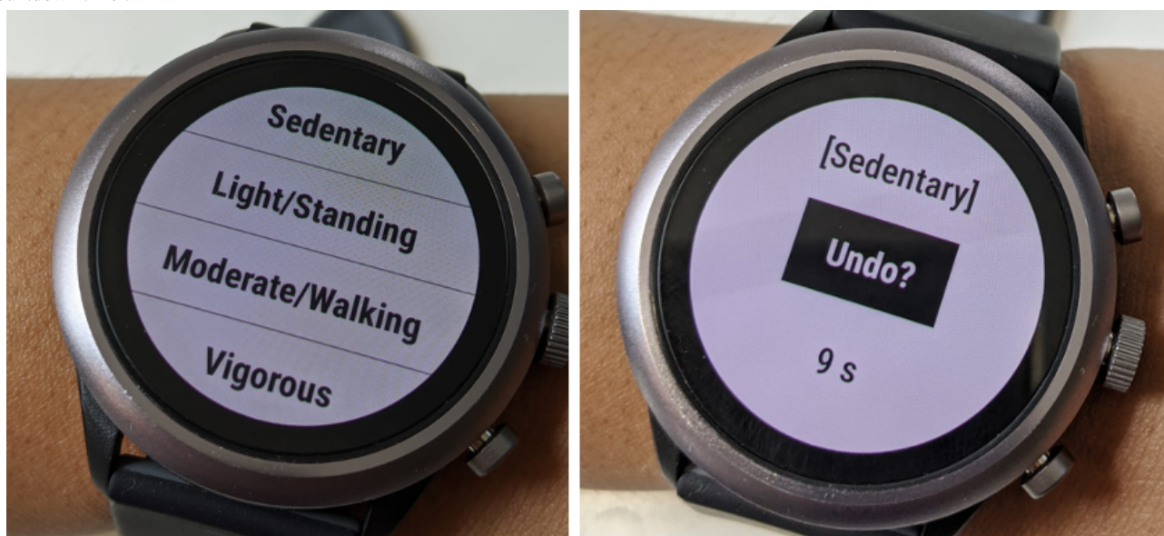
Figure 1. (Left) \mu EMA interface on a smartwatch with four activity intensity options. (Right) Undo screen to change response, available for 10 s, with a countdown timer.
