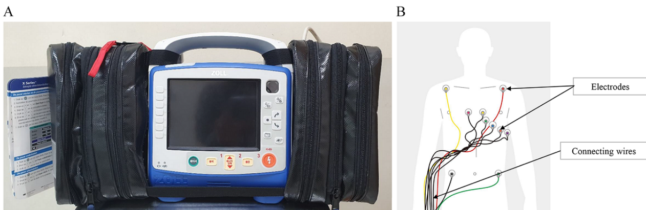
Figure 1. (A) The conventional 12-lead electrocardiogram device used for the control condition (X-series, ZOLL Medical, Chelmsford, MA, USA). (B) Attachment of electrodes on the patient’s body surface, which are connected to the main device.
