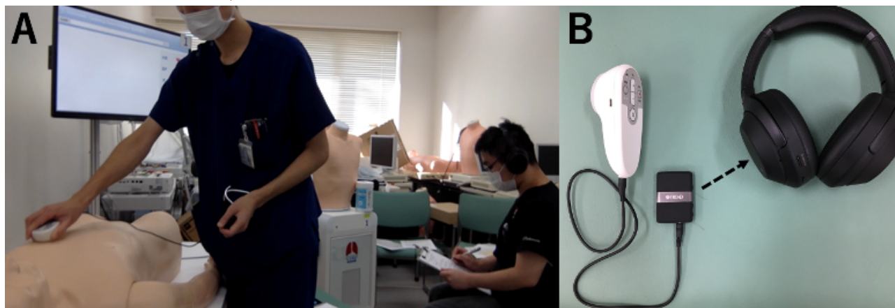
Figure 2. The remote auscultation processes: (A) The researcher is on the left, placing the electronic stethoscope on the cardiac patient simulator, and the participant is on the right listening to the cardiac sounds via a wireless, noise-canceling, stereo headset and Bluetooth transmitter; (B) the remote auscultation equipment including an electronic stethoscope; wireless, noise-canceling, stereo headset; and Bluetooth transmitter (Bluetooth connection is indicated with a dashed double arrow).
