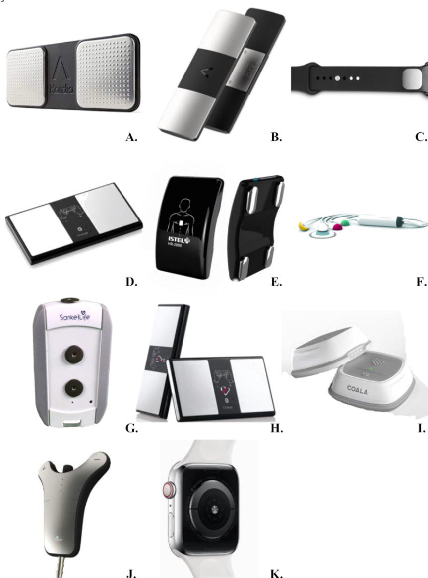
Figure 3. (A) Kardia Mobile (2 electrodes, 1-lead electrocardiogram). (B) Kardia Mobile 6L (3 electrodes, 6-lead electrocardiogram). (C) Kardia Band (2 electrodes, 1-lead electrocardiogram). (D) ECG Check (2 electrodes, 1-lead electrocardiogram). (E) Istel HR-2000 (4 electrodes, 6-lead electrocardiogram). (F) CardioSecur Pro (4 electrodes, 6-12-lead electrocardiogram). (G) Sanket Life-ECG, Stress, Fitness (3 electrodes, 1-12-lead electrocardiogram). (H) GEMS Mobile ECG for HeartCheck CardiBeat (2 electrodes, 1-lead electrocardiogram). (I) Coala Heart Monitor (3 electrodes, 2-lead electrocardiogram), J. i2Dtx for CardioSleeve (3 electrodes, 3-leads electrocardiogram). (K) Apple Watch Series 4 (3 electrodes, 1-lead electrocardiogram) [41-51].
