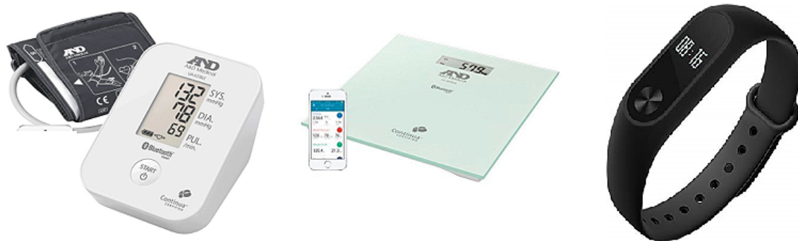
Figure 2. Bluetooth-enabled peripheral devices. From left to right: sphygmomanometer (A&D Medical UA-651BLE), weighing scale (A&D Medical UC-352BLE), and activity monitor (Xiaomi MiBand 2).
