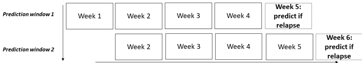
Figure 1. Sequential relapse prediction approach used in this study. Features are extracted from a period of 4 weeks to predict if a relapse might occur in the coming week.
