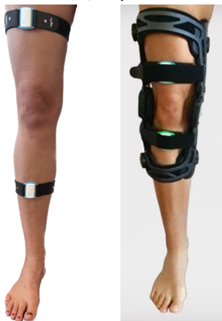
Figure 1. Re.flex technology directly attached to the lower limb (left) and Sporlastic GmbH GENUDYN OA SMART with re.flex technology (right).
