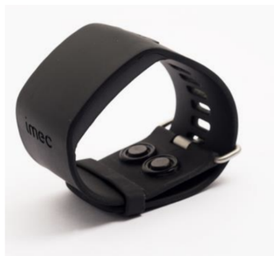
Figure 1. (A) Chest patch for gathering electrocardiogram and accelerometer and (B) wristband for gathering electrodermal activity, skin temperature, and accelerometer.
