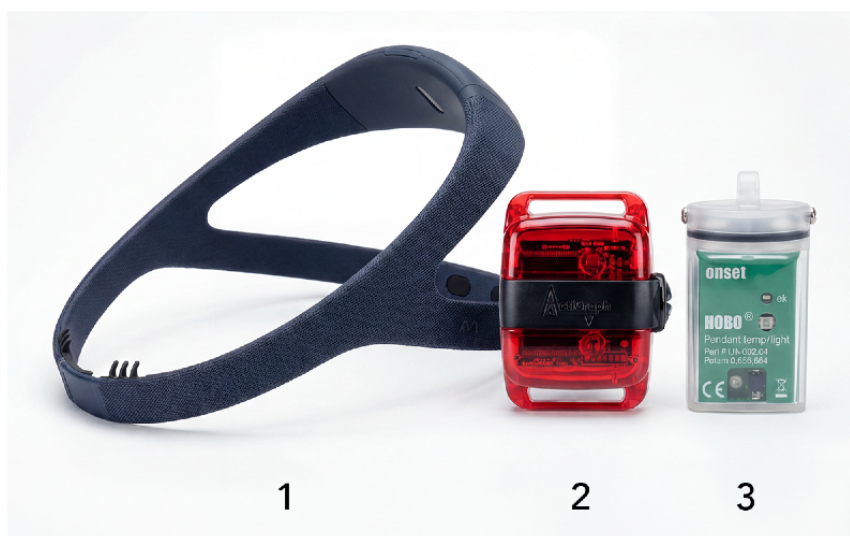
Figure 1. Study Sensors: (1) Dreem 3 Headband (Beacon Biosignals); (2) wGT3X+ triaxial accelerometer (ActiGraph); (3) HOBO Data Logger (Onset Computer Corporation).
