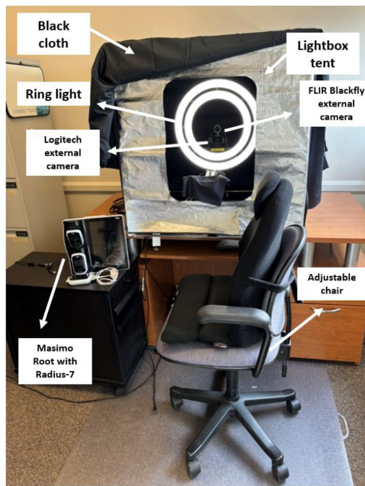
Figure 1. Hardware configuration of the data collection system at the research team’s laboratory.
